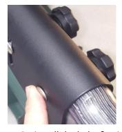
Re-install the bolts & raise the riser to approximate location & Press firmly on the bolt head while tightening the knob.
