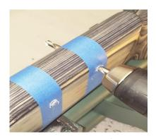
Finish up with the **1/4"** bit & drill all the way through
