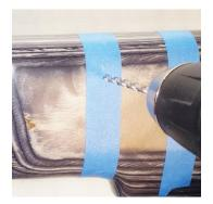
Use the **7/32"** bit first & drill half way through on all 4 dented marks, then all the way through
