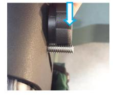
Place a knob on the side of the bolt & use a black sharpie to make a mark where the arrow is on the knob & Cut to length with a Dremel or Hacksaw. Round the bolts for proper fit
