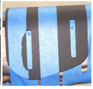
Depending on your stock, make a mark at the top of each slot as I could have done on this Boyd's Pro Varmint Stock. If your stock is narrower at the top of the comb use another transfer punch to space your marks evenly lower on the front slot only.
